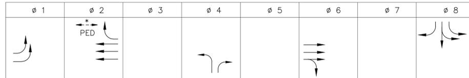
PROPOSED SEQUENCE AND TIMING FOR FULLY-ACTUATED CONTROL (ISOLATED)
