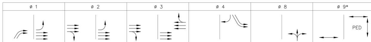
PROPOSED SEQUENCE AND TIMING FOR FULLY-ACTUATED CONTROL (ISOLATED)
