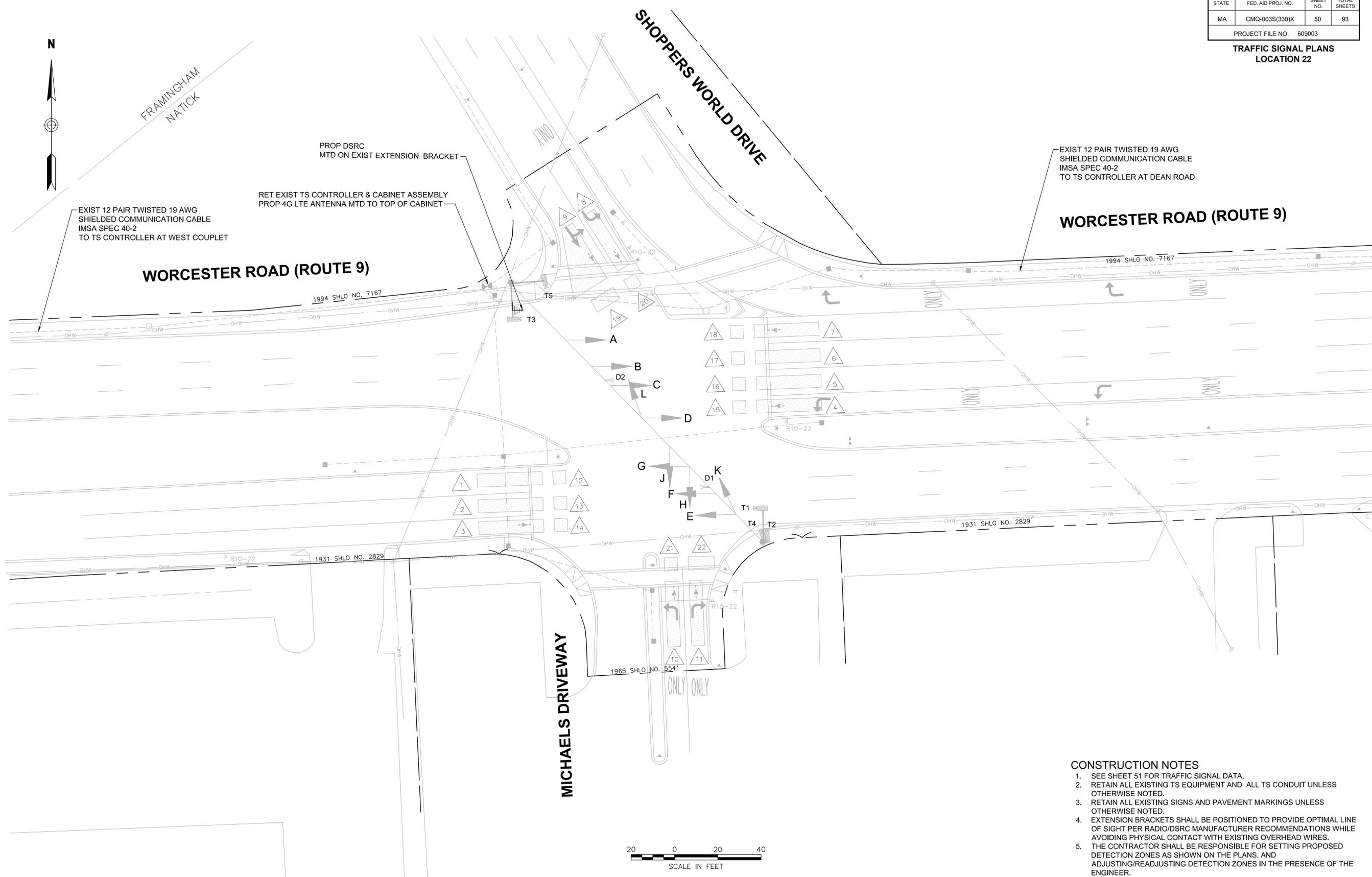
EXIST 12 PAIR TWISTED 19 AWG SHIELDED COMMUNICATION CABLE IMSA SPEC 40-2 TO TS CONTROLLER AT DEAN ROAD
