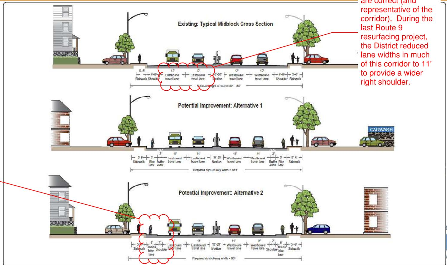
Recommend verifying that these dimensions are correct (and representative of the corridor). During the last Route 9 resurfacing project, the District reduced lane widths in much of this corridor to 11' to provide a wider right shoulder.
